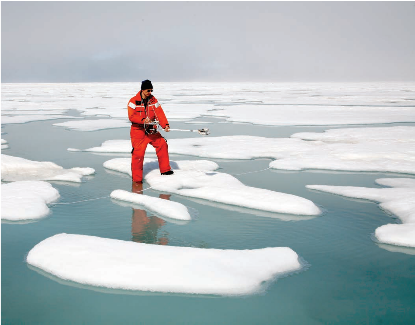
UAF scientist Dr. Chris Petrich takes measurements of total albedo over melting landfast sea ice at Barrow, Alaska. (UAF, James Barker)
